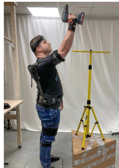
Figure 2: Task 1: Holding a power drill above the head
