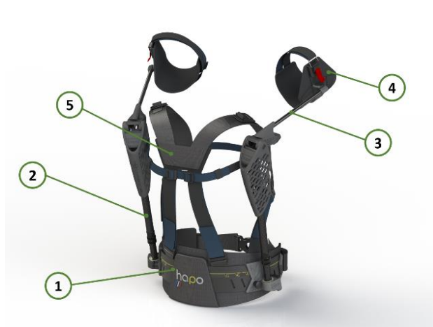
Figure 1: Exoskeleton HAPO UP, ErgoSanté, France. (1) Belt; (2) Mast; (3) Boom; (4) Interface; (5) Textile harness.
