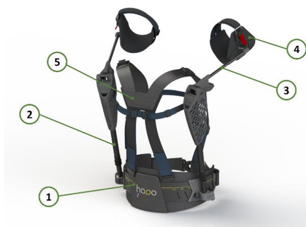
Figure 1 : Exosquelette HAPO UP, ErgoSanté, France. (1) Ceinture ; (2) Mât ; (3) Potence ; (4) Interface ; (5) Harnais textile.
